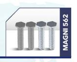
Magni 562 is a chrome-free duplex coating that combines electroplated zinc nickel and hex-chrome-free passivated substrate with an aluminum-rich organic topcoat. A coating that can be engineered to specific coefficient-of-friction needs, Magni 562 is offered with exempt solvents and typically applied to fasteners, including nuts, bolts and other hardware. Magni 562 can be applied via dip-spin or spray application methods.
