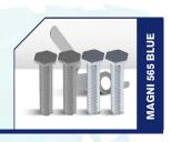
Magni 565 Blue is a chrome-free duplex coating that combines an inorganic zinc-rich basecoat with an aluminum-rich organic topcoat. Formulated as a two-coat system and resistant to automotive fuels and fluids, Magni 565 Blue is the preferred fastener coating of leading global automotive manufacturers. It provides superior corrosion protection and cost-effectiveness, and is typically applied to externally threaded fasteners, stampings and other hardware.
